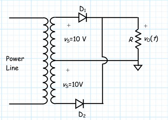
Conversely, if  $v_S$ =-10 V, the anode of  $D_1$  will be 10V **below** ground potential (i.e., -10V), while the anode of  $D_2$  will be 10V **above** ground potential:
