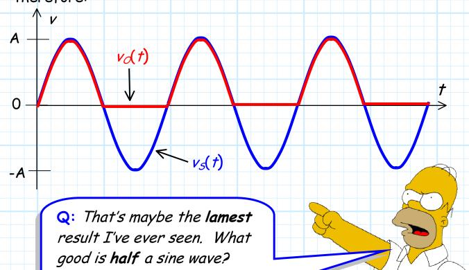
A: Although it may appear that our rectifier had little useful effect on the input signal  $v_s(t)$ , in fact the difference between input  $v_s(t)$  and output  $v_d(t)$  is both important and profound.
