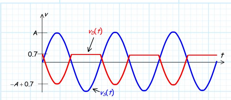
Note that this minimum diode voltage is very negative, with an absolute value ( $|v_D^{min}| = A - 0.7$ ), approximately equal to the value of the source magnitude A.
