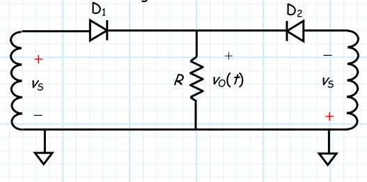
Note that the secondary voltages at either end of this circuit are the **same**, but have **opposite** polarity. As a result, if  $v_5$ =10, then the anode of diode  $D_1$  will be 10 V **above** ground, and the anode at diode  $D_2$  will be 10V **below** ground—just like before!
