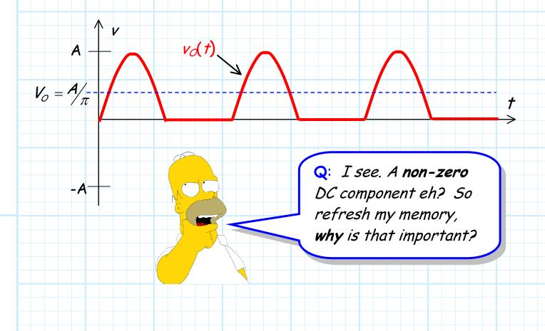
A: Recall that the power distribution system we use is an AC system. The source voltage  $v_s(t)$  that we get when we plug our "power cord" into the wall socket is a 60 Hz sinewave—a source with a zero DC component!
