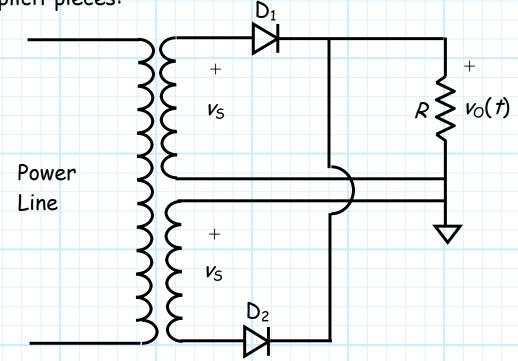
We will now ignore the primary winding of the transformer and redraw the remaining circuit as:
