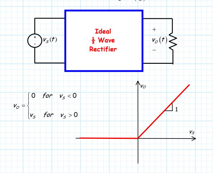
Pretty simple! When the input is negative, the output is zero, whereas when the input is positive, the output is the same as the input.
