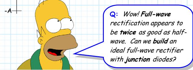
A: Although we cannot build an ideal full-wave rectifier with junction diodes, we can build full-wave rectifiers that are very close to ideal with junction diodes!
