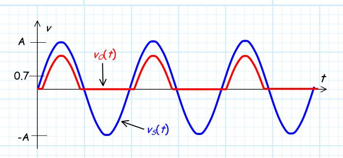
Although the output is **shifted downward** by 0.7 V (note in the plot above this is **exaggerated**, typically A >> 0.7V), it should be apparent that the **output** signal  $v_{\mathcal{S}}(t)$ , unlike the input signal  $v_{\mathcal{S}}(t)$ , has a **non-zero** (positive) **DC** component.
