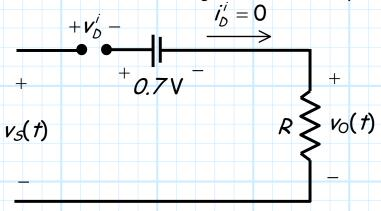
Q: Fascinating! The output voltage is **zero** when the ideal diode is reverse biased. But, precisely when **is** the ideal diode reverse biased? For **what** values of  $v_5$  does this occur?
